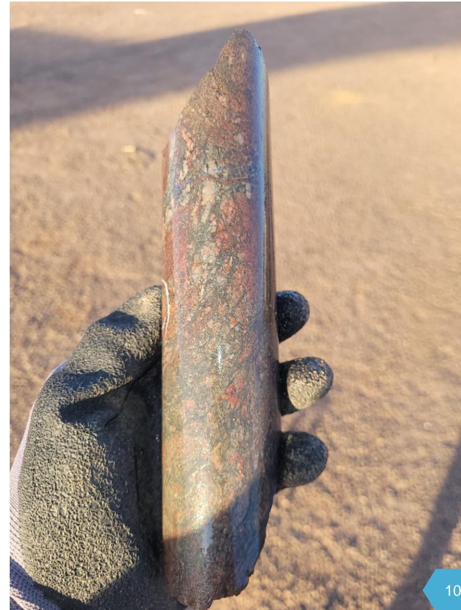
Photo of diamond core from Hole DD03 – Uranium mineralisation in altered fault breccia 252.9m
