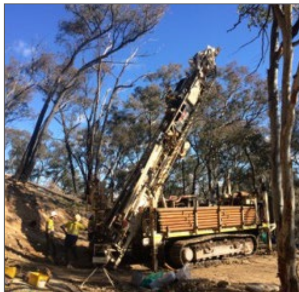
Figure 1: RC drill rig in operation at the Main Ridge Prospect, located within the Basin Creek Project, NSW.
