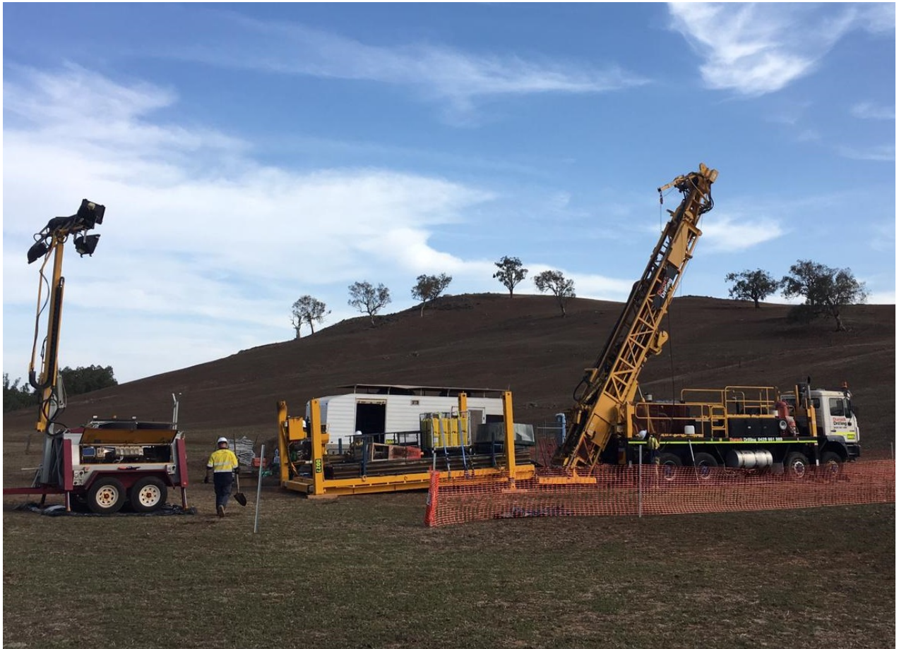
Figure 2: Diamond drill rig mobilised on site at the Junee Copper-Gold Project, NSW.
