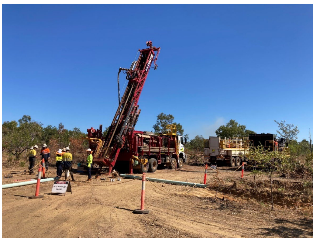
Figure 1: RC drilling underway at Nabarlek Uranium Project (NT)
