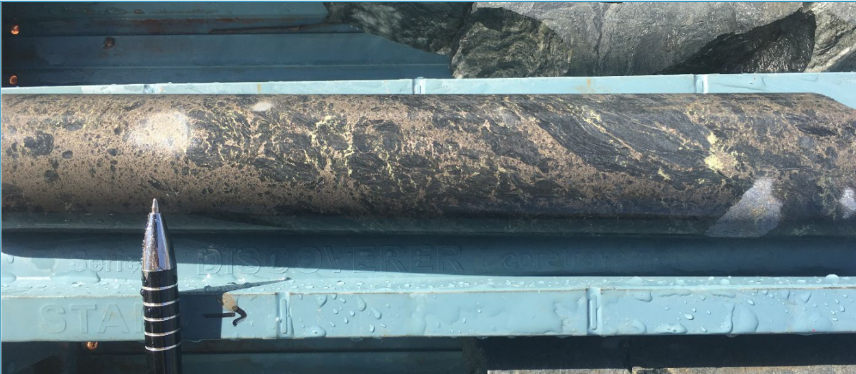
Semi massive pyrrhotite with chalcopyrite from 551.6m (Hole 20WD001). Gold mineralization is also associated with the copper.
