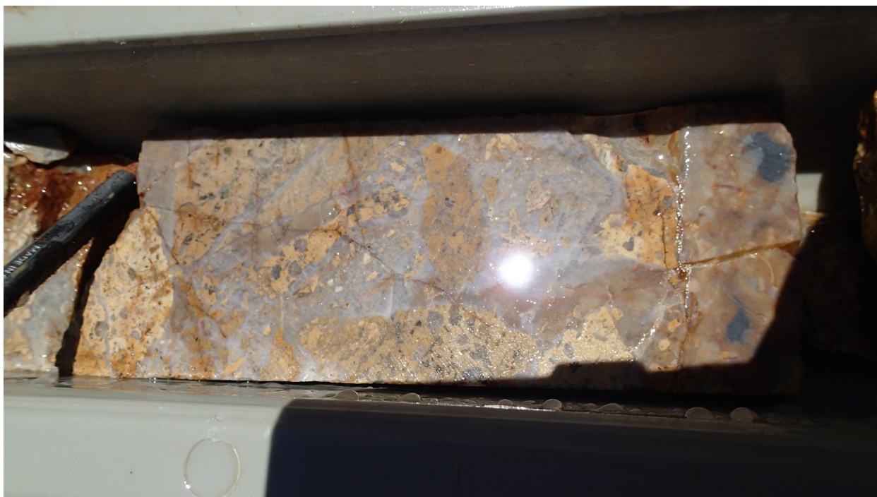
Photo 1: Drill core from DDH 1, 12 to 13m showing quartz veins and brecciation. Intervals assays 1m @ 6.2g/t Au from 12m.
