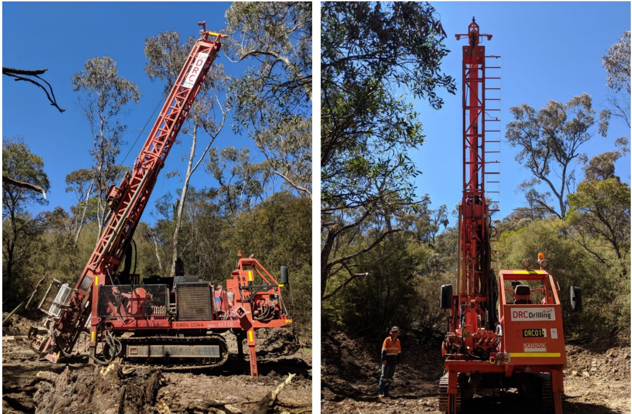
Figure 4: Diamond drill rig setting up at Bogong on Hole 1, line 6081600mN
